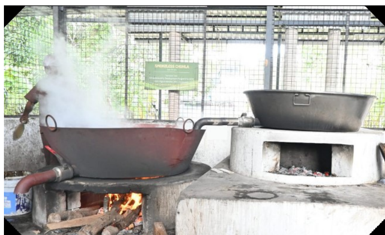
Eco-Friendly Smokeless Chulhas Supporting Sugarcane Juice Pre-Heating and Concentration, Extracting Juice with electric crusher and Releasing Bagasse
